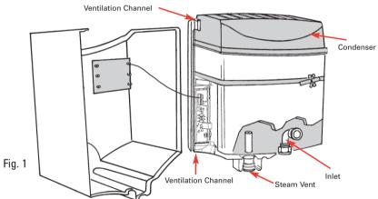
The unit must be connected to cold, mains fed, drinking water only. Pressure range between 0.7 Bar/69kPa (10psi) and 10.0 Bar/940kPa (140psi).
